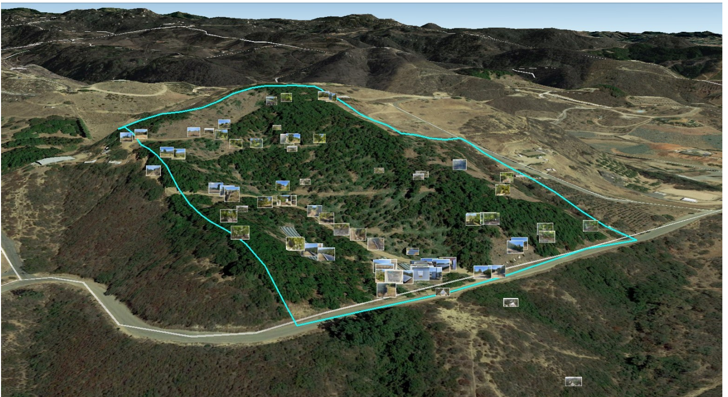
Exhibit 1: Ground and drone images pinned on an orthomosaic layer in Google Earth
